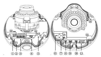
Internal interface of HD network zoom (non-) IF dome camera-V2.0
