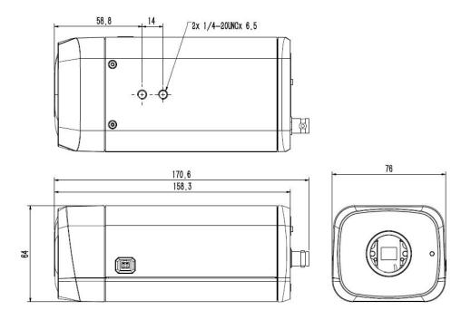
Dimensions of HD Network Gun Camera - V3.0
