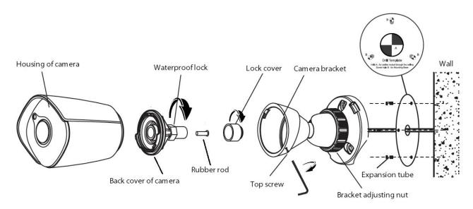
Installation Diagram of HD Network IR Integrated Machine (MINI) -V2.0
