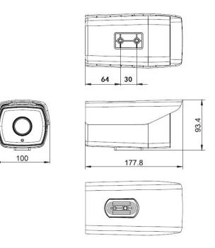
Dimensions of HD Network IR Integrated Machine - V2.0
