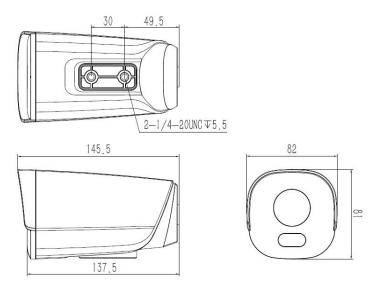
Dimensions of HD Network IR Integrated Machine - V4.0 (without integrated support)
