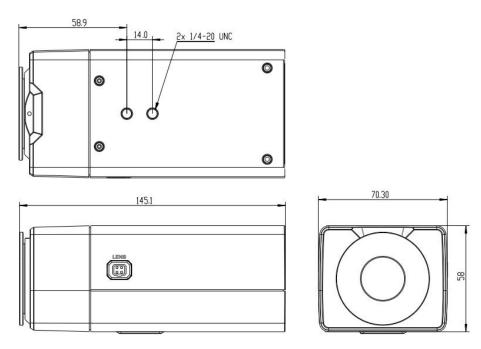
Dimensions of HD Network Gun Camera - V1.0/V2.0
