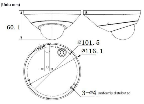
Dimensions of HD Network Special-shaped Safe IR Dome Camera
