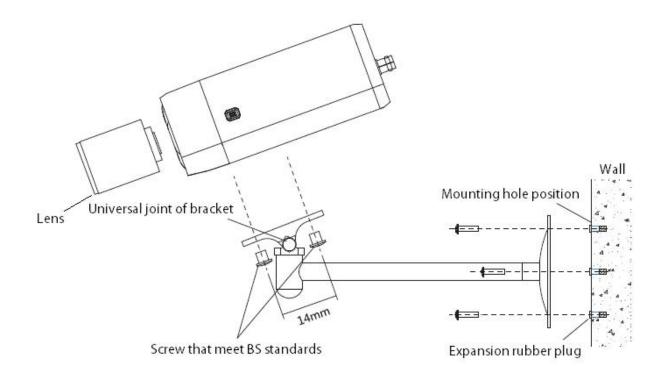
Installation Diagram of HD Network Gun Camera
