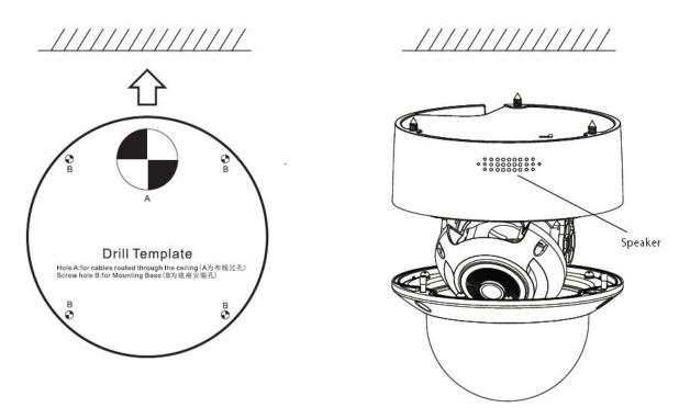
Installation Diagram of HD Network Zoom IR Dome Camera-V3.0peaker
