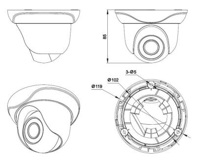
Dimensions of HD Network IR Dome Camera (MINI)
