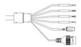
Alarm output (ALARM\_OUT A/ALARM\_OUT B) Alarm input (ALARM\_IN1/ALARM\_IN2/GND) Audio interface (AUDIO\_IN/AUDIO\_OUT/GND) RS485 (A/B) Power interface
