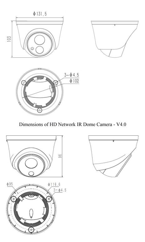
Dimensions of HD Network IR Dome Camera - V5.0
