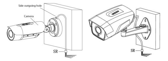
Installation Diagram of Tail Cable
